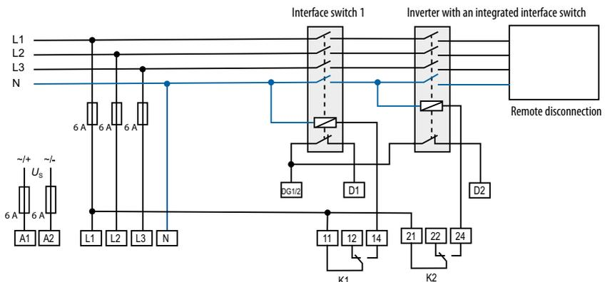
**Wiring diagram VDE-AR-N 4110:2018-11 – basic program 4110 (suggestion)**
