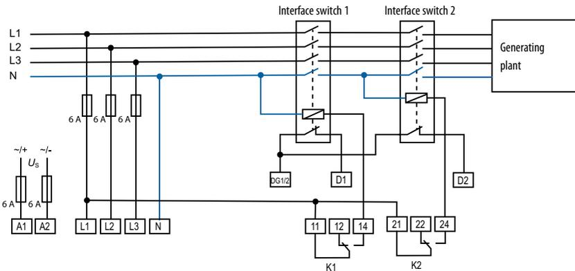
Further wiring diagrams in the manual.
