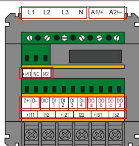
Overview of the terminals: The connections are located on the back of the device.
