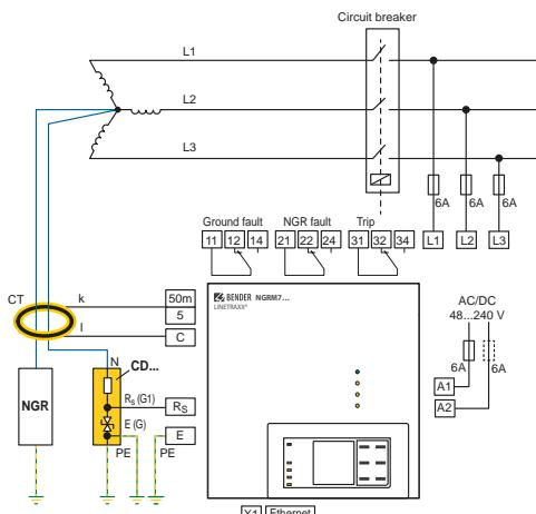
**i** The "N" connection of the CD-series coupling device should be as close to the transformer star point as possible.
