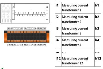
Cable lengths of the measuring current transformers Ĭ Install the measuring current transformers according to the instructions in the respective data sheet of the measuring current transformer. When connecting, observe the maximum cable lengths.
