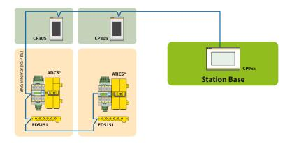
In the example, the ICU is monitored from the station base via BMS bus.
