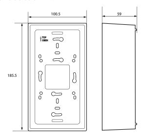
Any clearance between the surface-mounting enclosure and the wall must be compensated using washers. Never tighten the screws with a cordless screwdriver; only do so by hand. If this is disregarded, the surface-mounted housing can become warped.
