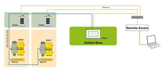
In the example, the ICU can be monitored from the station base. In addition, remote maintenance is possible via the building services or Bender.
